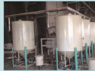
Oil-adding Machine in Feed Line
